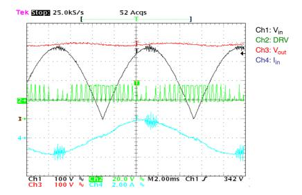
Figure 5. The Waveforms at 265 Vac, 300 W as Controlled by 200 kHz NCP1654
