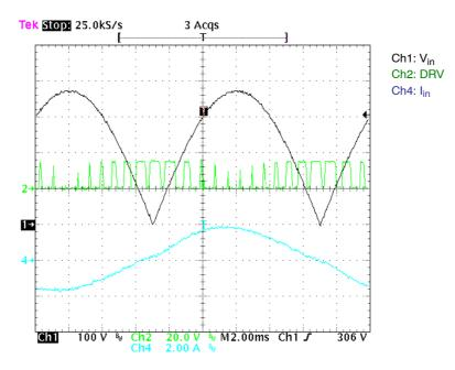
Figure 7. The Waveforms after Modifying the  $V_{\mbox{\scriptsize M}}$  Pin Structure
