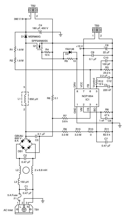
Figure 8. 300 W Application Schematic
