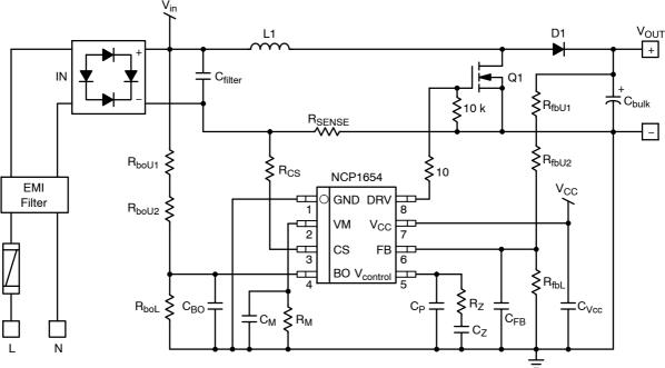
Figure 1. PFC STAGE DIMENSIONING – Generic Schematic
