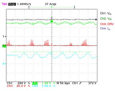
Figure 4. Zoom-in with Waveforms at Peak of 265 Vac
