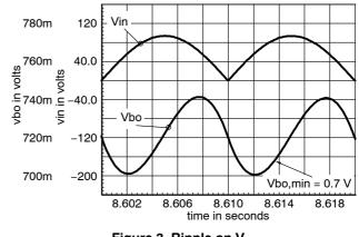
Figure 3. Ripple on V<sub>bo</sub>
